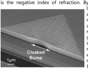
Optical "carpet" cloak based on nanostructured silicon.
