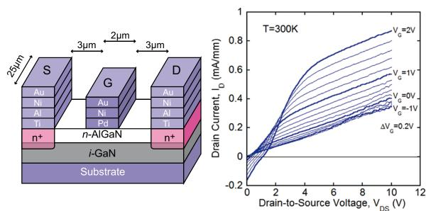
*Fig. 3: Schematic drawing of a cubic GaN/AlGaN field effect transistor (left) and its output character-istics (right).*
