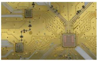
Ceramic board with analog-to-digital converters and "syn-QPSK" signal processing component.
