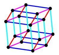
Projection of a hypercube with 16 optical "synQPSK" symbols in the 4-dimensional space of two quadratures and two polarizations onto a 2-dimensional plane.
