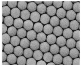
SEM top-view of a nanosphere lithography mask. Nanoobjects can be formed in the open spaces between each triple of spheres.
