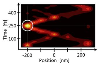
*If the pulse excites a quantum wire, the electrons are concentrated at a desired location in space and time.*
