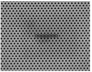
*Photonic crystal cavity in GaAs with embedded InAsquantum dots.*
