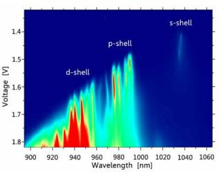
Intentionally positioned quantum dot embedded in a pin-junction.
