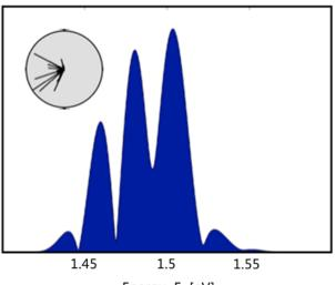
Energy E [eV] Spectrum of a laser pulse with the respective phases found by an optimization routine.
