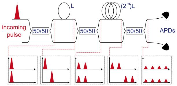
Experimental setup for photon statistics measurement.
