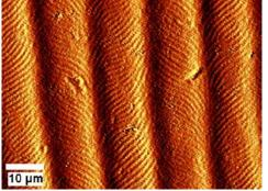
But also dissipative structures caused by electroconvection can be utilized for fabricating regular microstructures: The figure to the left shows the surface shape of a polymer film (detected by atomic force microscopy), where a transient pattern induced by a uniform electric field was permanently imprinted into the polymer surface by means of photopolymerization. The lattice constant of the chevrons is smaller than 1 micrometer.
