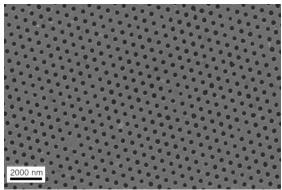
to be useful e.g. for (biomimetic) antireflection coatings, as substrates for the localized growth of novel semiconductor nanostructures such as nanodots and nanowires and for the growth of high-quality semiconductor thin films in materials systems with a large crystalline lattice mismatch (nano-heteroepitaxy).
