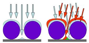
Cross-sectional view of nanosphere lithography beads used as masks in deposition processes.
