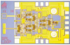
magnetic loop and electric dipole double probe integrated with switchable matched common source and common gate broad band amplifiers.
