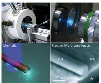
and large radiation enhancement of *Plasmonic nanolaser with emission at 490nm*.
