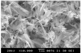
is studied in a collaboration with the group Prof. Lischka and As, aiming to reduce crystalline defects by the use of nanopatterned substrates. The growth of ZnO nanowires and nanoflakes by means of the vapour-liquid-solid mechanism in a gradient furnace is investigated in order to control the formation of this high-potential optoelectronic material.
