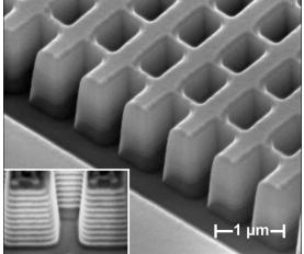
Metamaterial with a negative index of refraction.
