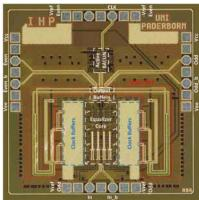
Based on first demonstrators at 10 Gbit/s and 20 Gbit/s in GaAs HEMT technology, a further improved concept was implemented in a 0.13  $\mu$ m SiGe HBT technology. Test circuits operating up to 110 Gbit/s input data rate have been demonstrated.
