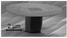
Low-threshold microdisk laser.
