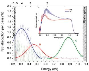
Fig. 1: Transmission spectrum in the THz range of the GaN/ AlGaN cubic QWs at 4.2K for TM- (red solid line) and TEabsorptions in cubic GaN/AIN quantum (blue dotted line) polarized light. ISB absorption is peaked
