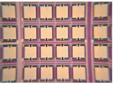
Micro mirror array for optical applications.
