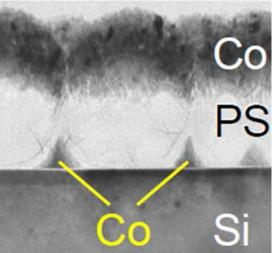
Cross-sectional TEM micrograph of a polystyrene (PS) mask on silicon, covered with cobalt to create Co nanopyramids.
