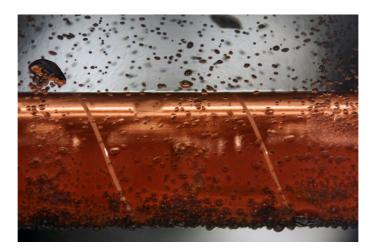
Figure 4.1.44: Boiling of FC-3284 on the structure A432 at p=1 bar,  $q = 40 \text{ kW/m}^2$ .
