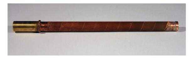
Figure 3.1.4: Photo of the test tube A428, provided with microstructure.
