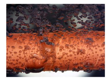
Figure 4.1.46: Boiling of FC-3284 on A425 at p = 0.5 bar, q = 3 kW/m<sup>2</sup>.
