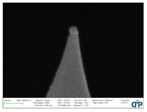
Figure S 10: TiO<sub>2</sub> coated tip used in this study after DFS measurements.
