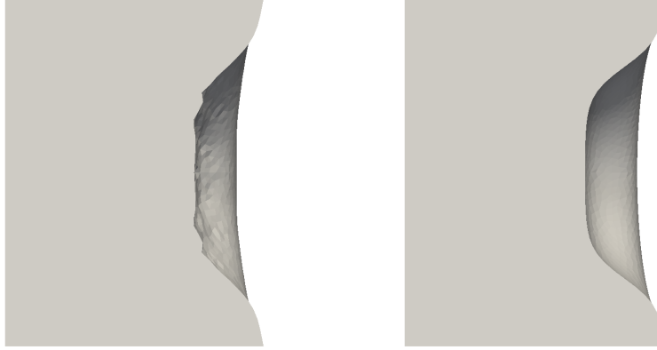
Figure 5.8: Cross-sectional comparison between reconstructed bump after 373 optimization steps and target bump.
