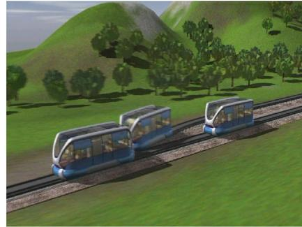
(b) Build-up of a Convoy of Three RailCabs at a Switch [NBP]
