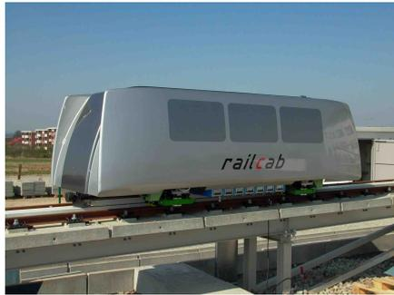
(a) RailCab Prototype in Scale 1:2.5 on Test Track
